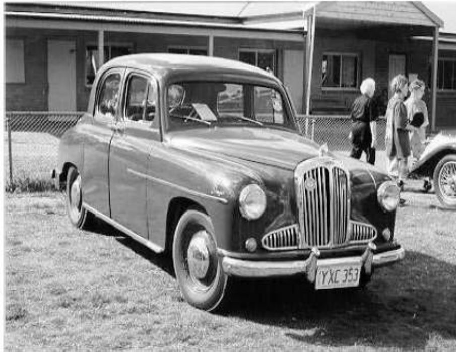
1954 Singer Hunter - GRP bonnet and side valences ( Source: The American Singer Owners Club )
