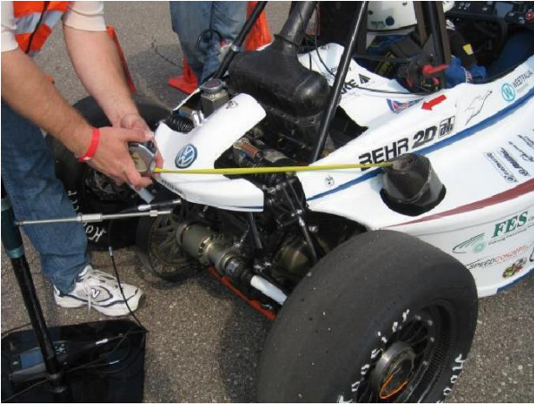
NOISE TEST LOCATION
